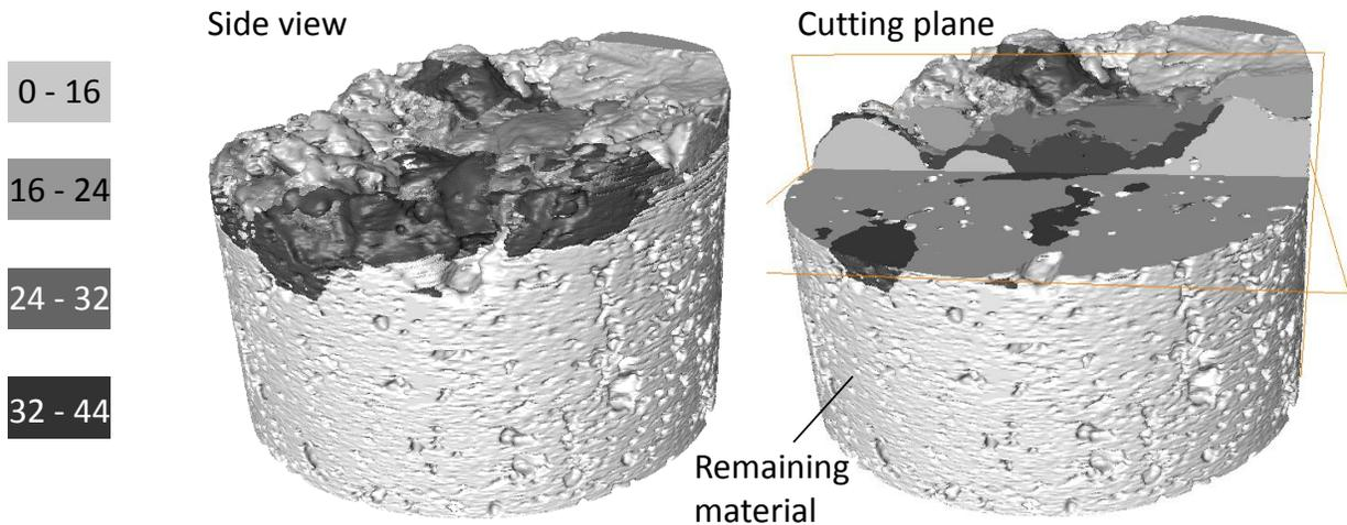
**Figure 14 – This model shows the material that has left the surface of the sample in different shades of gray. A cross section is shown in the second image. It shows that the materials are leaving in layers from the outside surface of the sample.**
