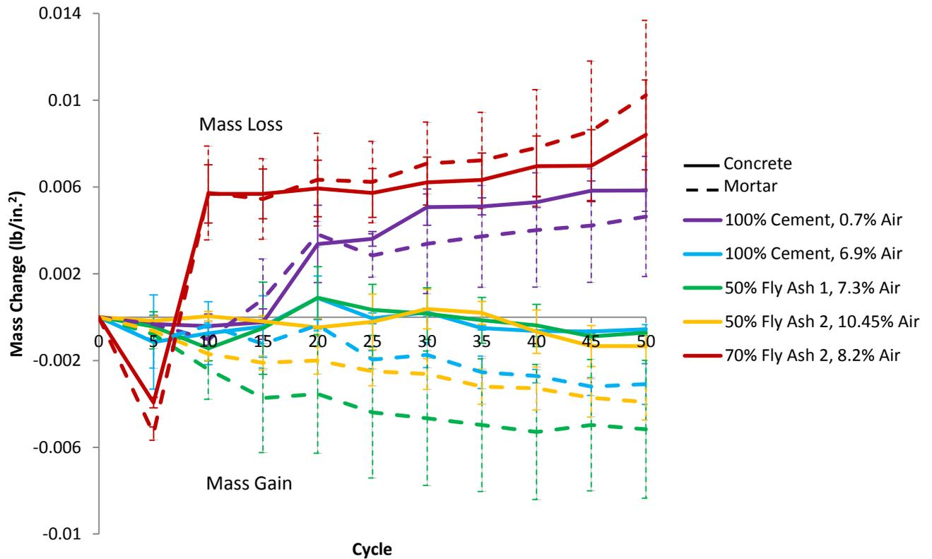
Figure 1 – Mass change for the concrete and mortar samples with freeze thaw cycles. A solid line corresponds to a concrete sample and a dashed line is a mortar sample.
