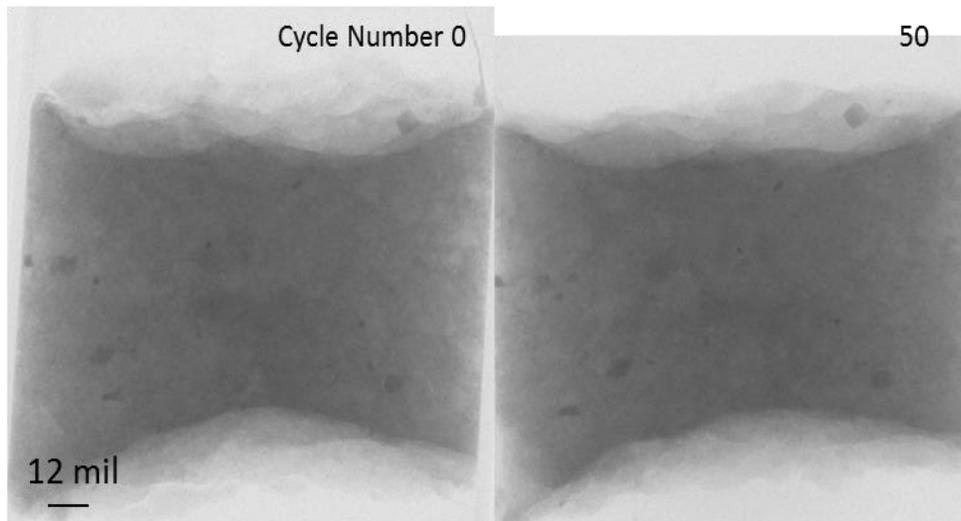
**Figure 8 - A sample with 50% Fly ash 2 and 10.45% air content that is 3/16" in diameter. The sample shows very little damage over 50 cycles.**
