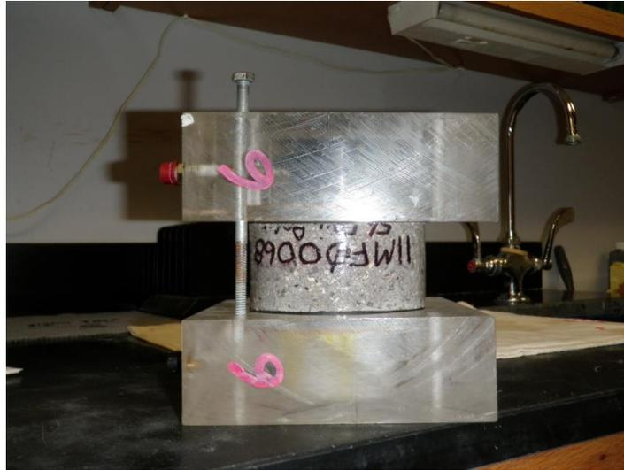
Figure 3 – Completed Rapid Chloride Specimen
