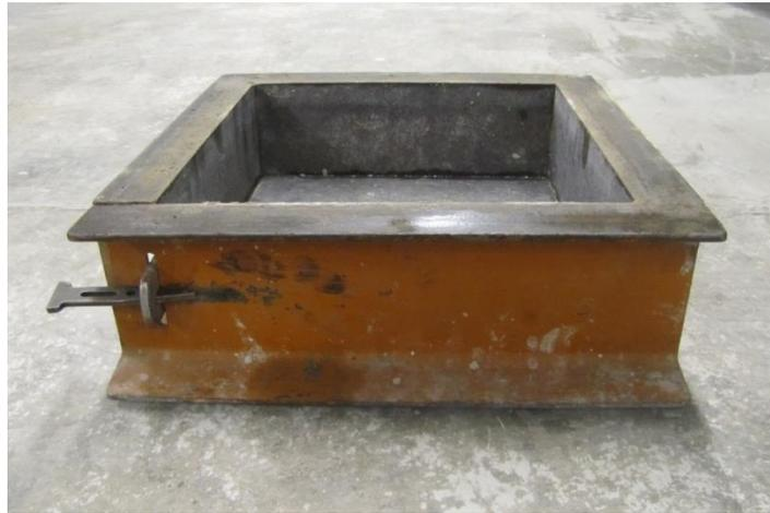
Figure 6 – Scaling Specimen Form
