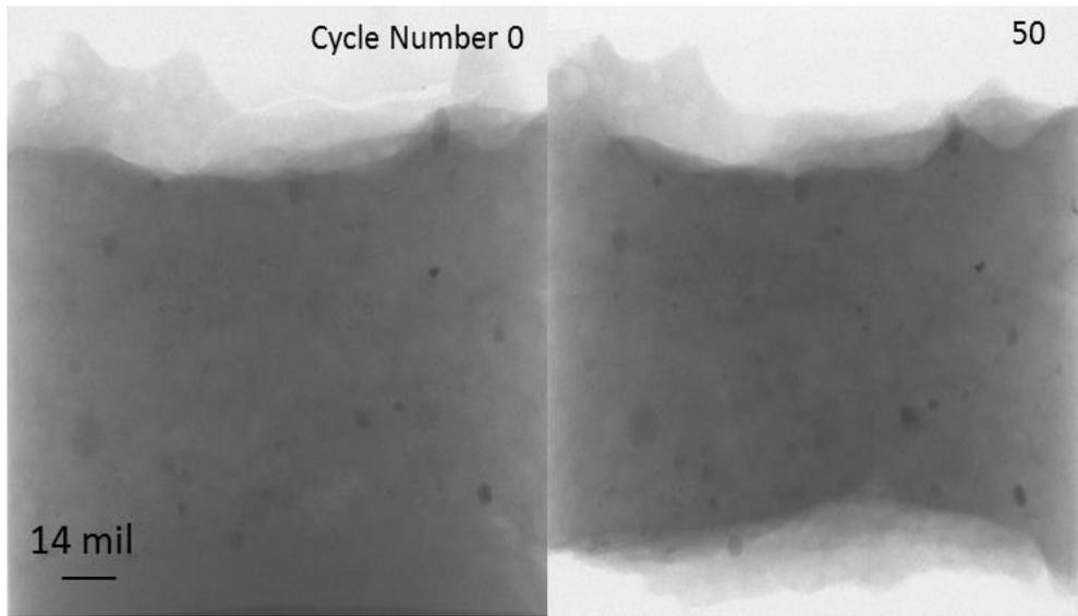
**Figure 3 – A sample of 100% cement and 0.7% air from the same mixture as the one shown in Fig. 2. This sample has 5/16" diameter and the damage is much less.**
