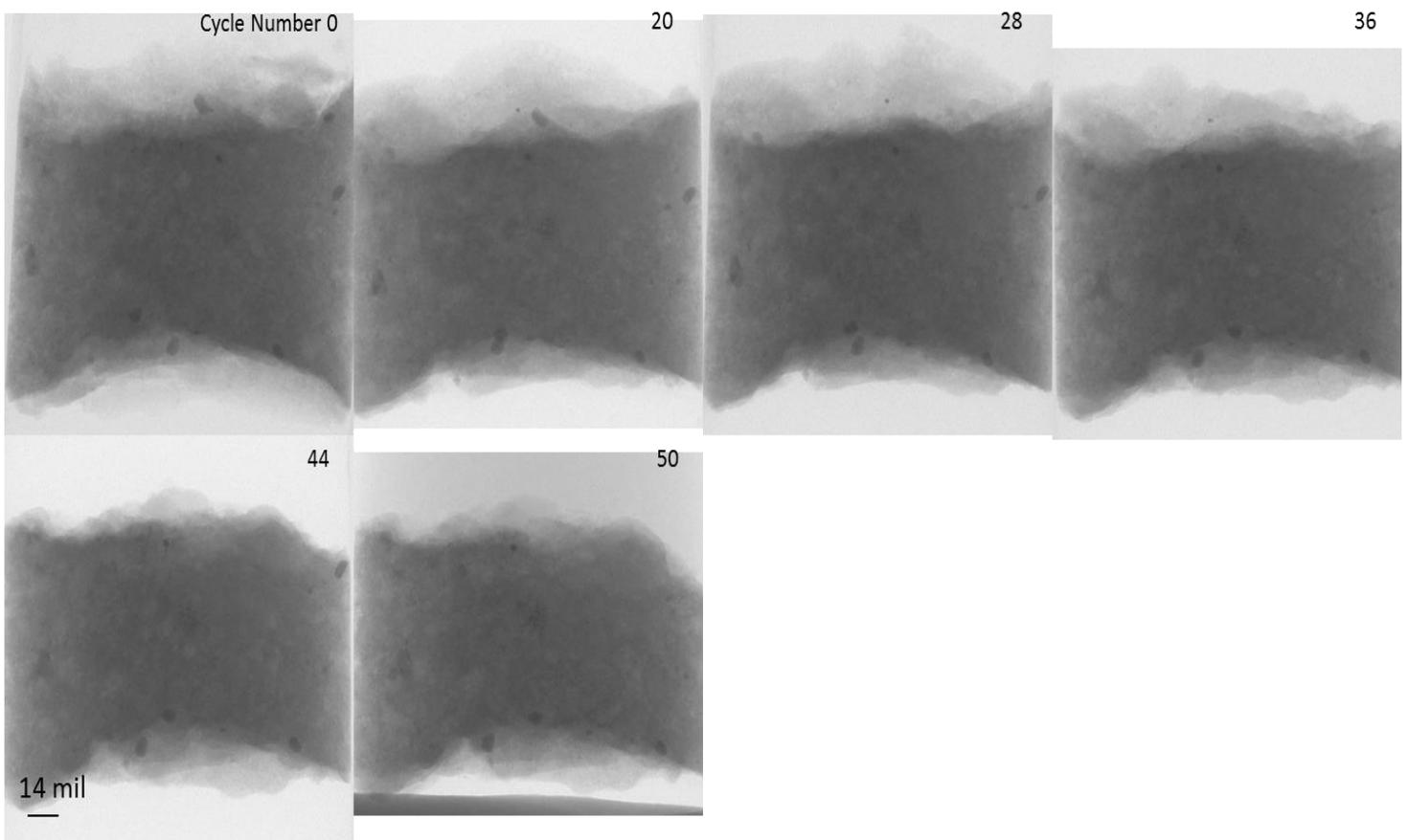
**Figure 9 - A sample with 50% Fly ash 2 and 10.45% air content that is 5/16" in diameter. The sample is the same as Figure 8 and shows moderate damage over the 50 cycles.**
