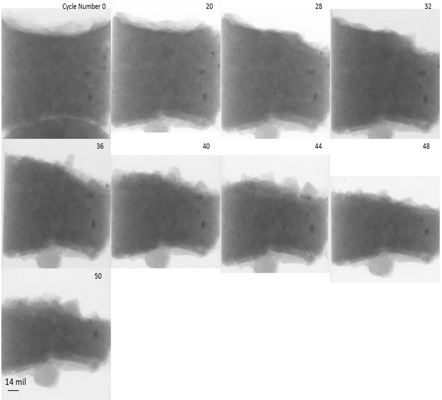
**Figure 5 - A sample with 100% cement and 6.9% air content that is 5/16" in diameter showing progressive damage over the 50 cycles. This is the same sample as in Fig. 4 but it has a larger diameter.**
