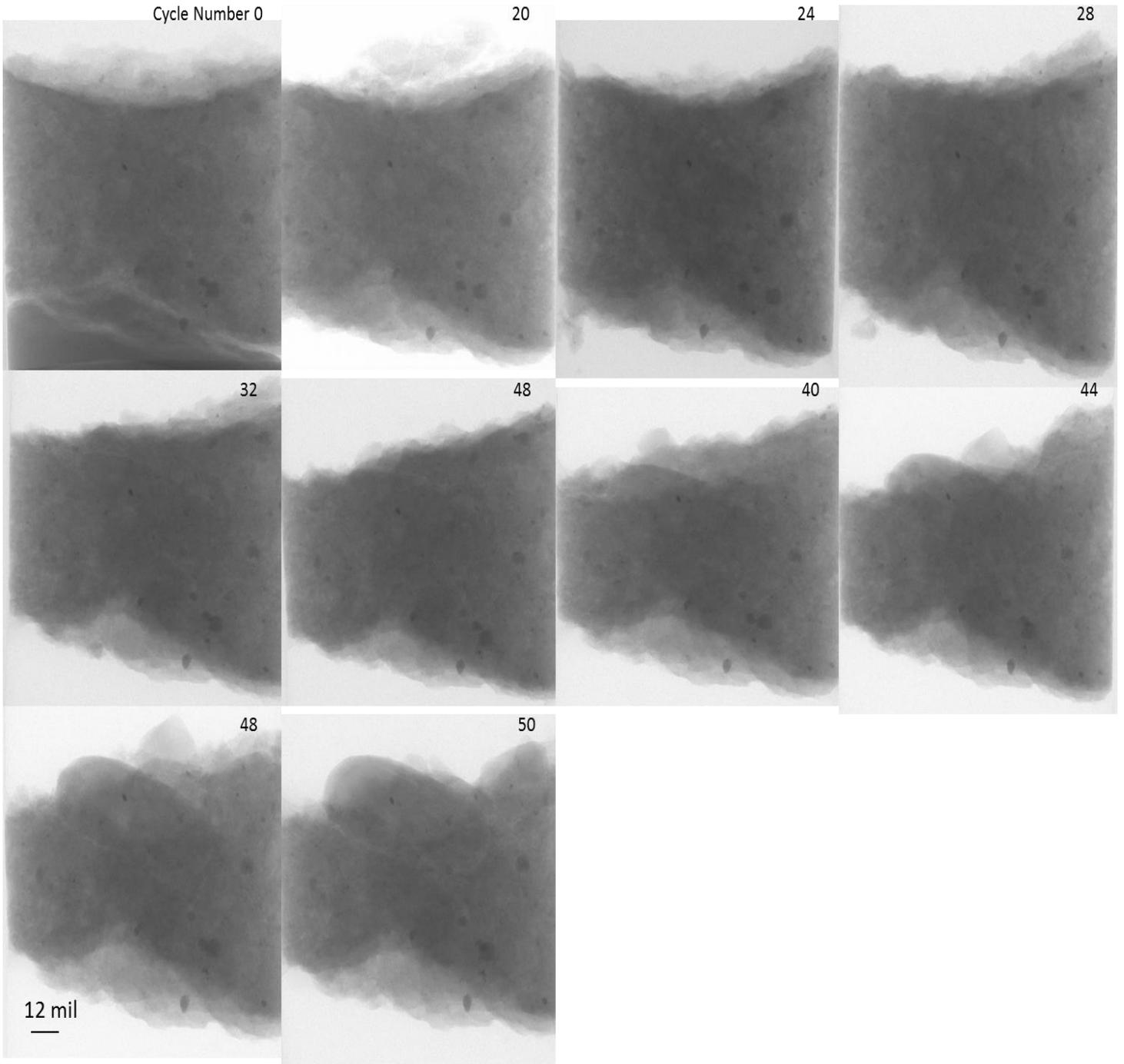
**Figure 7 – A sample with 50% Fly ash 1 and 7.3% air content that is 5/16" in diameter. This is the same sample as in Fig. 6 only it has a larger diameter and is showing increased damage.**
