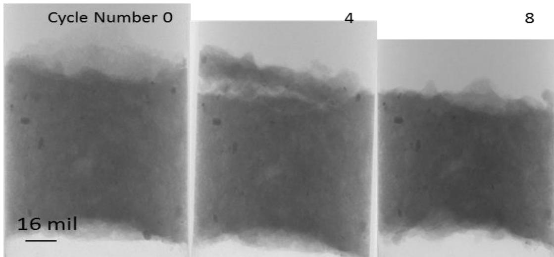
**Figure 11 - A sample with 70% Fly ash 2 and 8.2% air content that is 5/16" in diameter. This is the same material as is shown in Fig. 10. Again a different failure mode is observed then the other samples investigated.**
