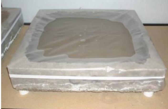
Figure 5 – Ponding Test Specimen
