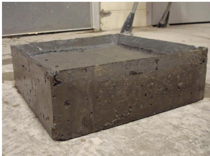
Figure 7 – Salt Scaling Specimen
