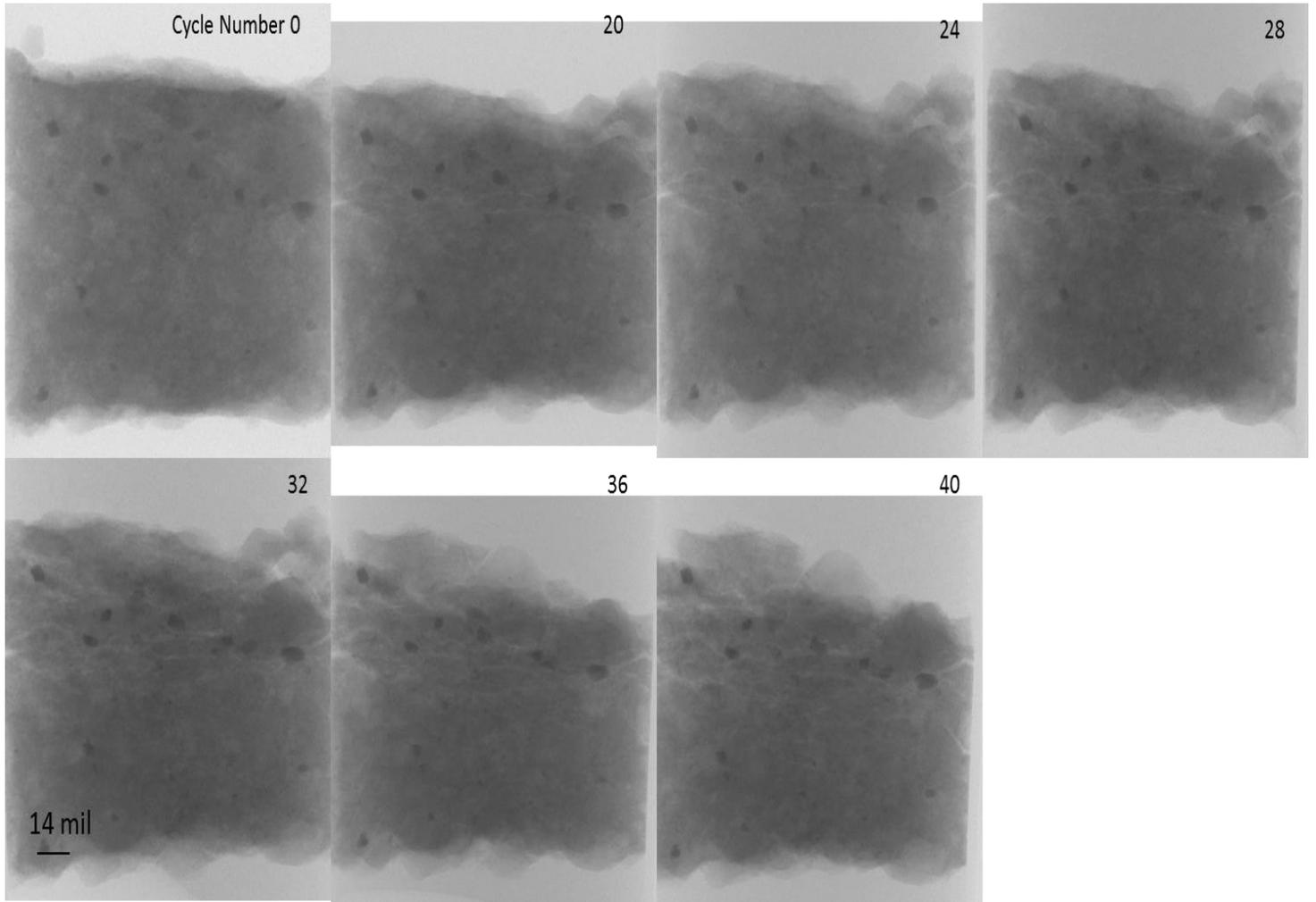
**Figure 10 – A sample with 70% Fly ash 2 and 8.2% air content that is 3/16” in diameter. The sample shows a different failure mode than the other samples investigated.**
