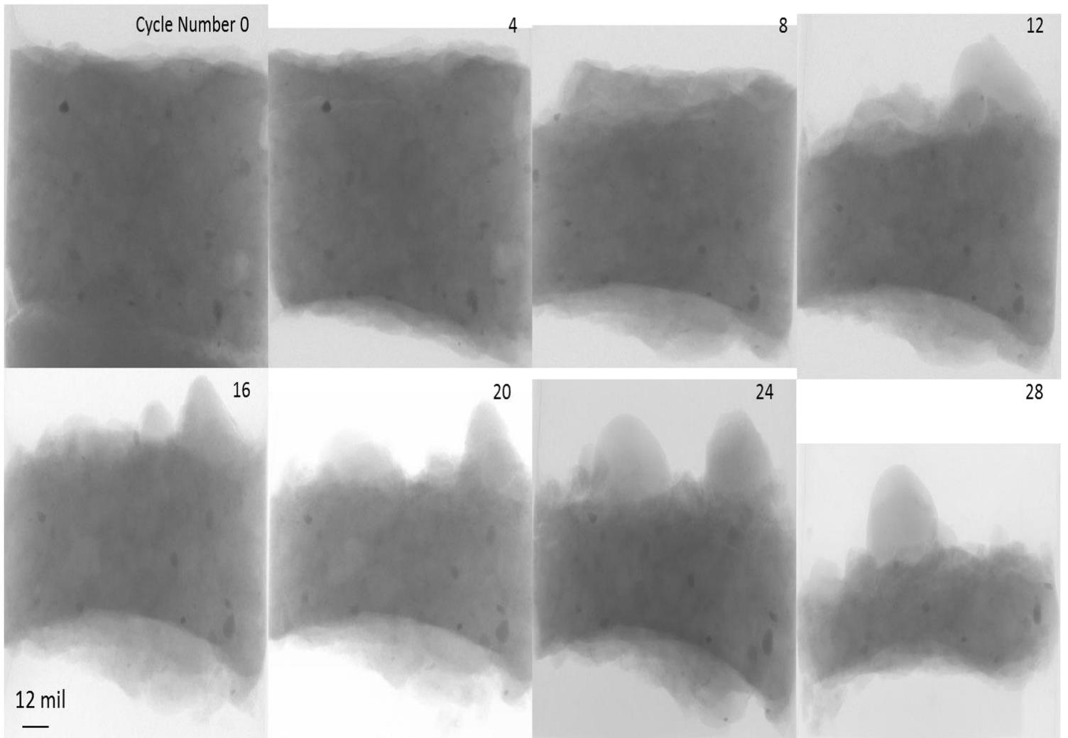
**Figure 2 – A 3/16" diameter sample with 100% cement and 0.7% air content.**
