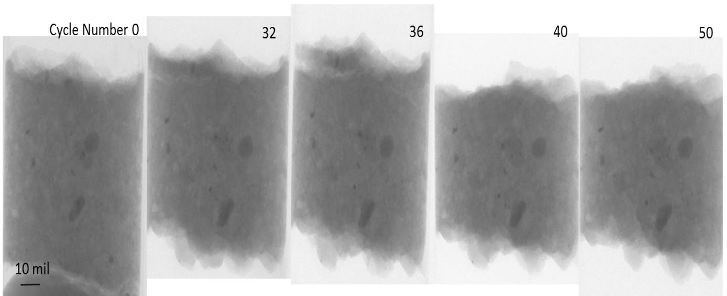
**Figure 6 - A sample with 50% Fly ash 1 and 7.3% air content that is 3/16" in diameter showing limited damage over the 50 cycles.**
