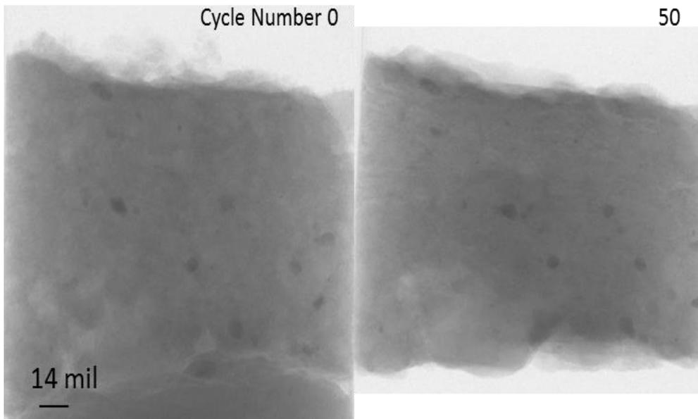
**Figure 4 – A sample with 100% cement and 6.9% air content that is 3/16" in diameter showing very little damage over the 50 cycles.**
