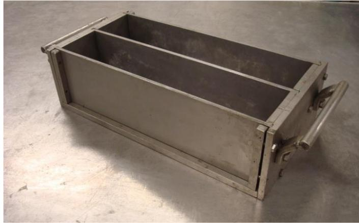
Figure 1 – Freezing and Thawing Specimen Molds
