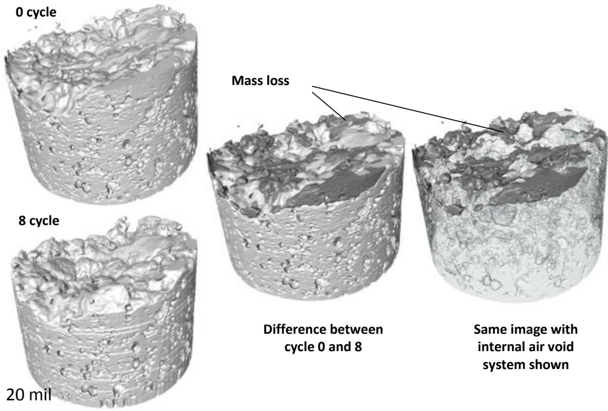
**Figure 12 – An overview of the tomography analysis between two cycles. The 3D models of the sample at zero and eight freeze thaw cycles. In the middle image a 3D model is shown with the material that has scaled off the sample shown in a darker color. The image on the far right shows the same sample with the internal air void system.**
