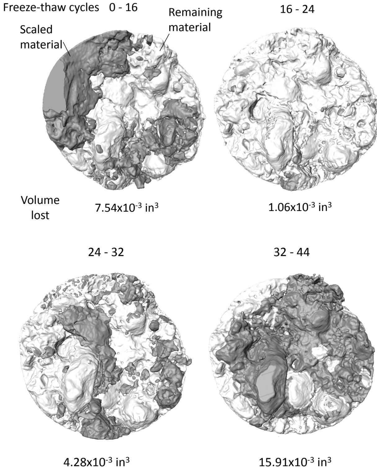
**Figure 13 – 3D tomography of the top surface of the samples showing how they change over different freeze-thaw cycles. The volume loss is also shown below each of the samples.**
