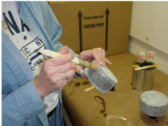
Figure 2 – Application of Setting Coating
