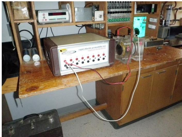
Figure 4 – Rapid Chloride Ion Test Setup
